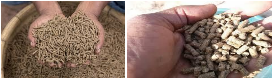
Fig. 6. The dried extruded fish feed using the fish feed extruding machine.
