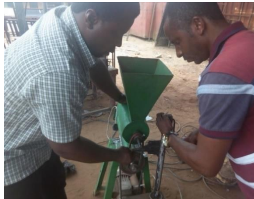
Fig. 5 Assembly Process for the Fish Feed Extruding Machine ongoing in the Workshop.
